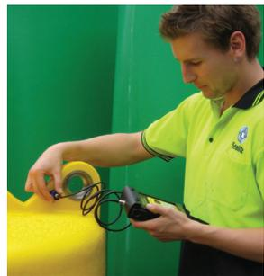
Ultrasonic testing ensures consistency of wall thickness in key areas such as mooring points.
