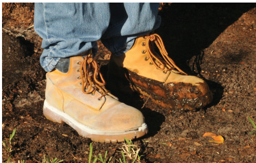
MUD TEST: Untreated boot (R) and boot sprayed with Ultra-Ever Dry (L). (Video available - See Back)
