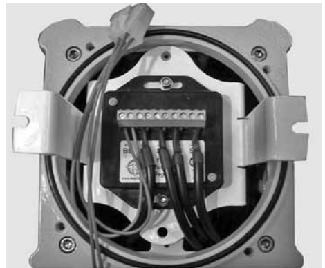
SL10 AMP Regulator shown when correctly fitted
