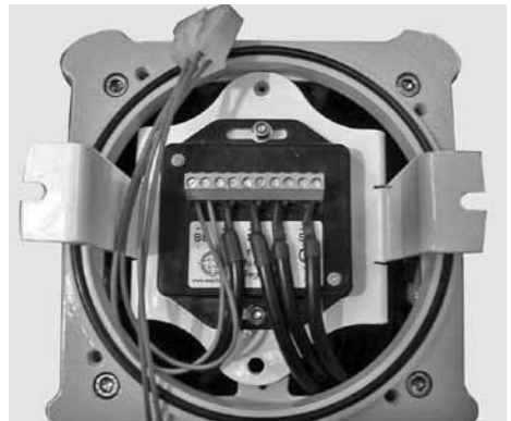
SL10 AMP Regulator shown when correctly fitted
