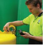
Ultrasonic testing ensures consistency of wall thickness in key areas such as mooring points.
