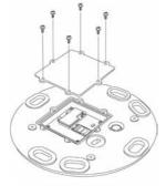
Remove the 6 retaining screws from the cover on the underside of the light, to gain access to the GSM compartment.
