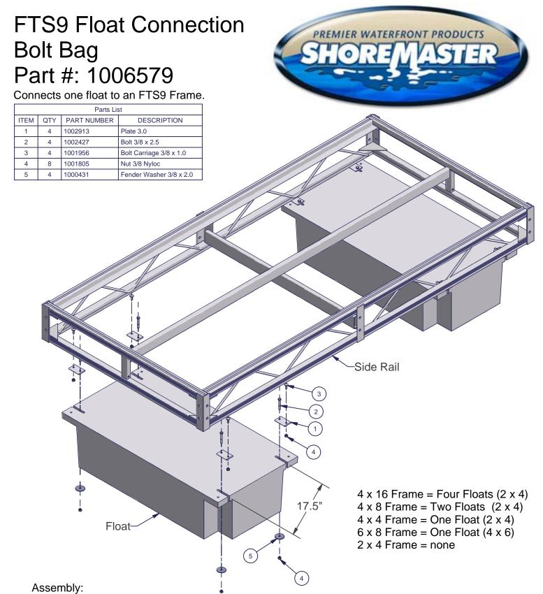
Attach two Plates 3.0 to each Side Rail with one Bolt Carriage 3/8 x 1.0 and one Nut 3/8 Nyloc at each place - as shown.
