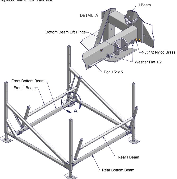
Attach the Rack to the Front I Beam with one Bolt 1/2 x 5, two Washers Flat 1/2 and one Nut 1/2 Nyloc Brass connecting the Rack Lift Hinge to the I Beam in two places - as shown.
