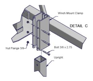
Slide Winch Mount onto Lift Side Winch Upright with the bolt holes facing the front of the lift Secure Winch Mount by using three Bolts 3/8 x 2.75 and three Nuts Flange 3/8 - as shown in Detail "C."
