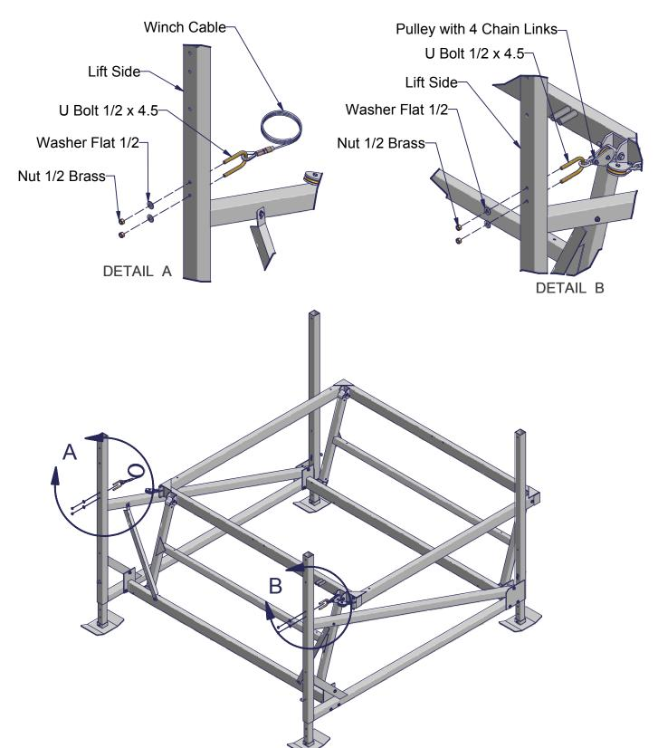
Route the Winch Cable through the two Pulleys with 3 Chain Links and the one Pulley with 4 Chain Links - as shown.
