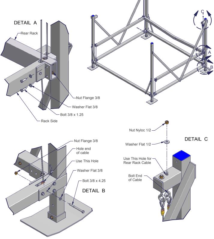
Set the Front Rack in place and attach to the Rack Sides. At each end secure with one Bolt  $3/8 \times 1.25$ , two Washers Flat 3/8 and one Nut Flange 3/8 in two places as shown in Detail "A."
