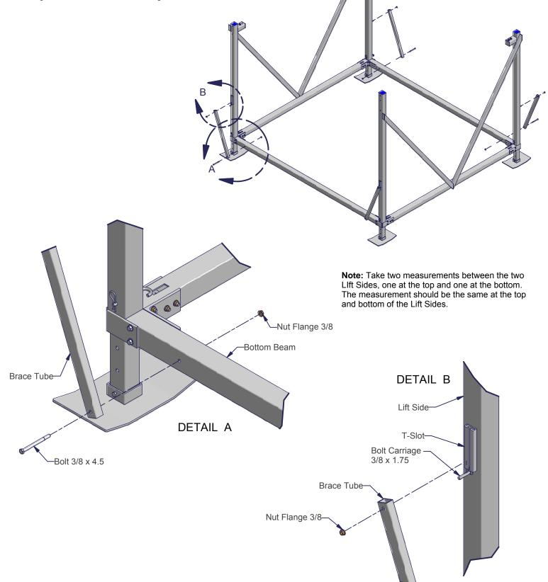
Place the Rack Sides in the Lift Sides as shown with Connection Angles facing out.
