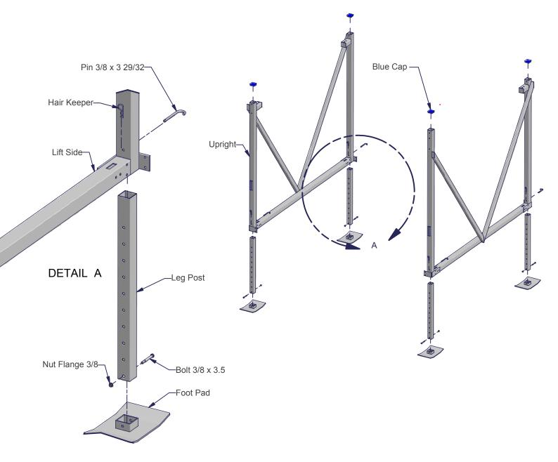
Attach one Bottom Beam to front both Lift Sides. Secure each end of the Bottom Beam with five Bolts 3/8 x 4.25, five Washers Flat 3/8 and five Nuts Flange 3/8 - as shown in Detail "A."
